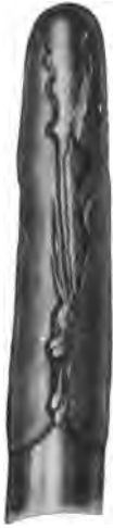
FIG. 352.—DEEPLY SCRATCHED WAX - TIPPED CATHETER. From impact against stones in pelvis of kidney. (Mrs. M. H., Gyn. No. 8639, April, 1901.) See four succeeding figures.
